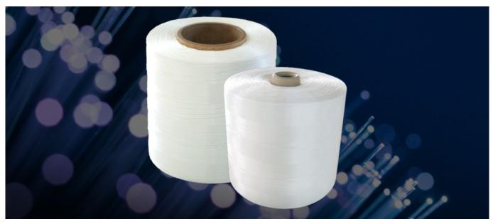
Our "swellable" solution against water penetration into your cables with unique swelling property of up to 50 times its own weight. Our most common grades are 1800 Deniers and 2500 Deniers and they can be placed either longitudinally, helically or used as binder yarns.
